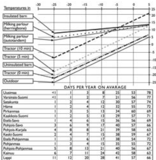
Fig 4. The dependence of temperatures in various workplaces in a farm on the outdoor temperature and the approximate number of days per temperature range recorded by various Labour and Trade Centres (TE Centres) of Finland.
